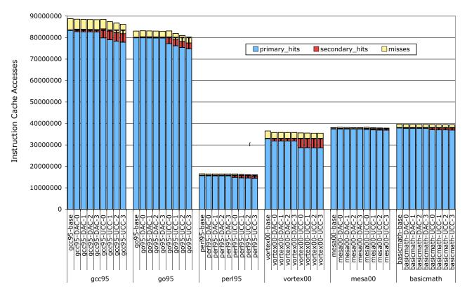
Figure 6.5. IL1 accesses distribution for 20 cycles L2 for a 2-way, 16KB, 8 instructions per block, instruction cache, for valid blocks latency
