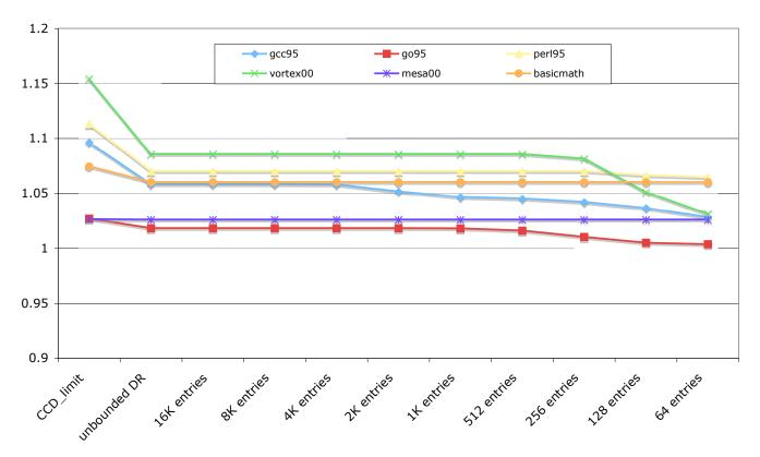
Figure 8.3. Performance potential of CATCH for a UCC with 128 entries in HDD and various sizes of DR
