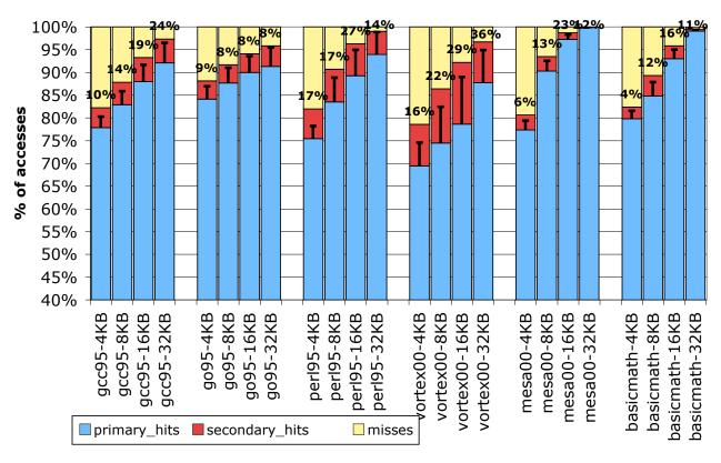
Figure 6.2. CCD for a 2-way, 8 instructions per block, instruction cache with UCC, for valid blocks
