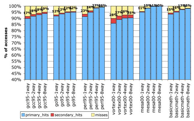
Figure 5.3. CCD for a 16KB, 8 instructions per block, instruction cache, for valid blocks
