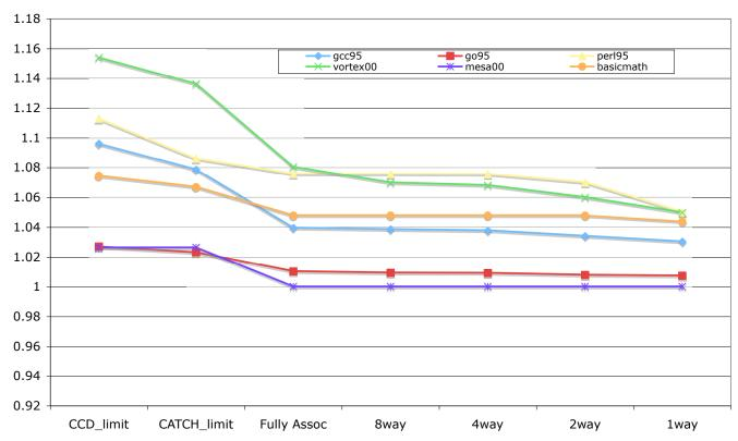
Figure 8.5. Effects of associativity on the DR with a 2-way HDD (128 entries HDD, 256 entries DR)
