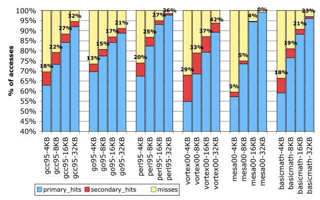
Figure 5.4. CCD for a 2-way, 4 instructions per block, basic block cache
