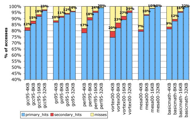
Figure 5.2. CCD for a 2-way, 8 instructions per block, instruction cache, for valid blocks
