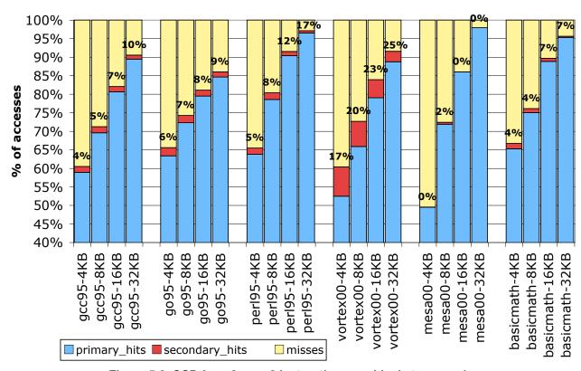
Figure 5.6. CCD for a 2-way, 8 instructions per block, trace cache
