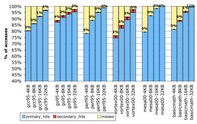
Figure 6.1. CCD for a 2-way, 8 instructions per block, instruction cache with UCC
