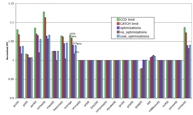
Figure 8.8. Effects of performance optimizations (4-way 256 entries DR, 2-way 128 entries HDD)
