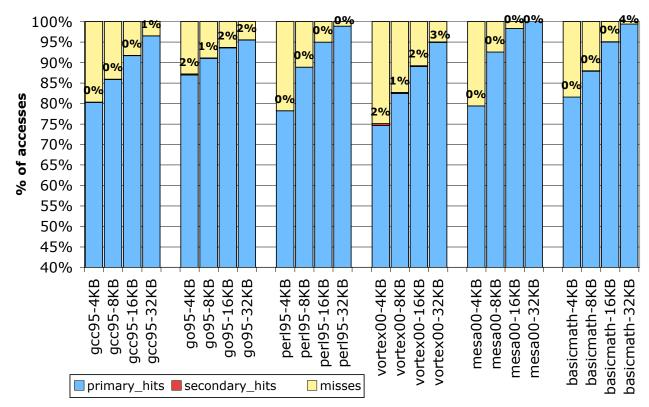
Figure 5.1. CCD for a 2-way, 8 instructions per block, instruction cache
