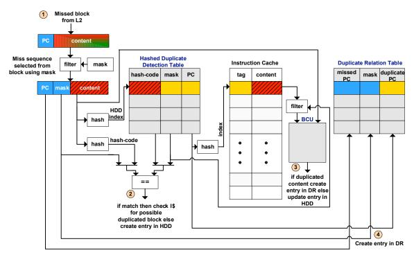
Figure 7.2. The flow with CATCH for a Cache miss, DR miss and HDD hit
