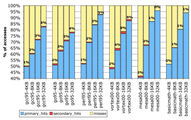
Figure 5.7. CCD for a 2-way, 16 instructions per block, trace cache
