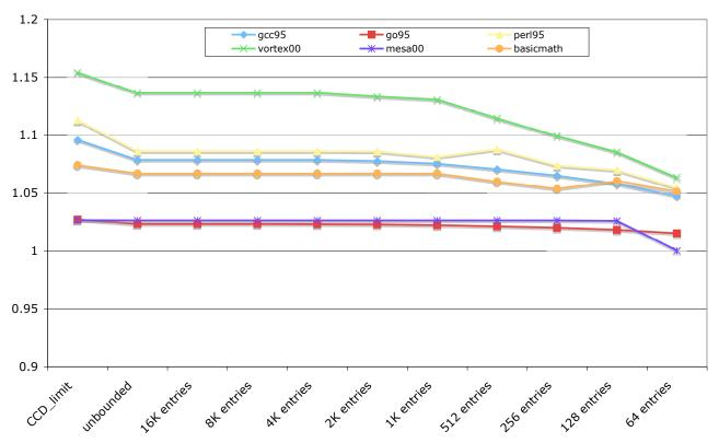
Figure 8.2. Performance potential of CATCH for a UCC using various sizes of HDD
