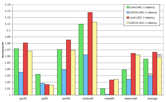
Figure 8.1. Performance potential of CATCH for DAC and UCC for 20 cycles L2 latency
