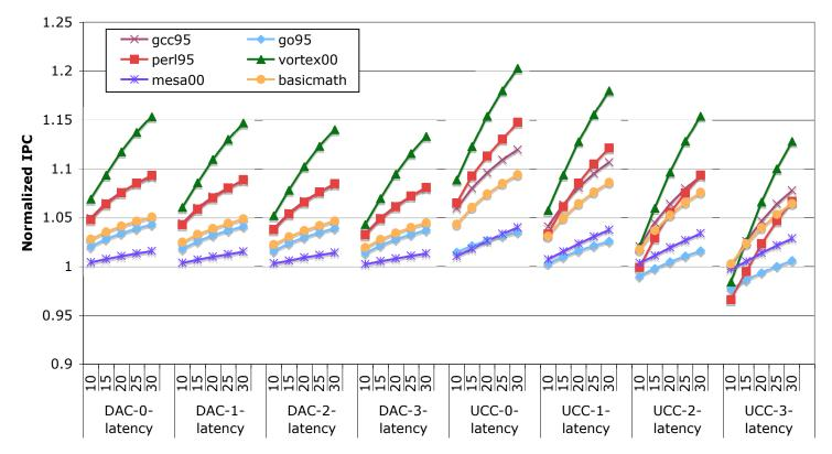
Figure 6.6. Performance potential of DAC and UCC for a 2-way, 16KB, 8 instructions per block, instruction cache, for valid blocks (Normalized IPC)
