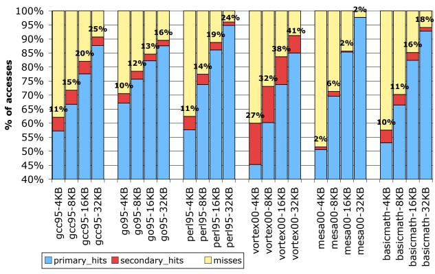
Figure 5.5. CCD for a 2-way, 8 instructions per block, basic block cache
